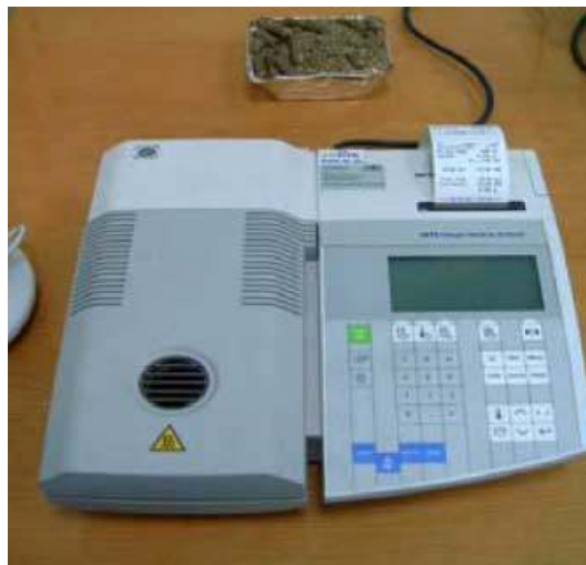
Fig. 2. HR 73 type moisture content-measuring instrument
