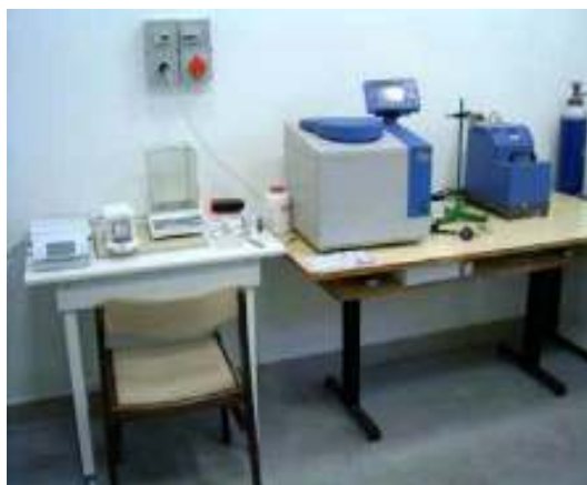
Fig. 3. IKA, C 2000 type combustion heat and heating value measuring appliance
