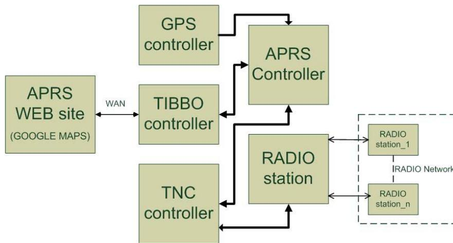
Figure 1. APRS node controller project structure
