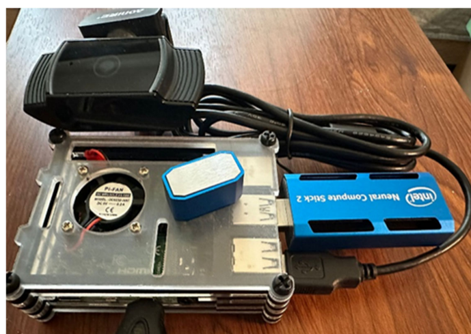
Figure 1. Used hardware components (Raspberry Pi 4B, NCS 2, USB camera).
