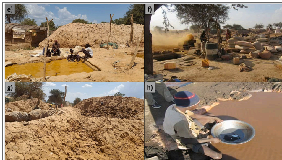
Fig. 11. Gold extraction practices in ASGM areas (a: miners around a small artificial pool filled with water for ore washing and panning; b: breaking rocks generates dust clouds; c: improper waste disposal; d: manual amalgamation of gold using mercury in a pan filled with muddy water).
