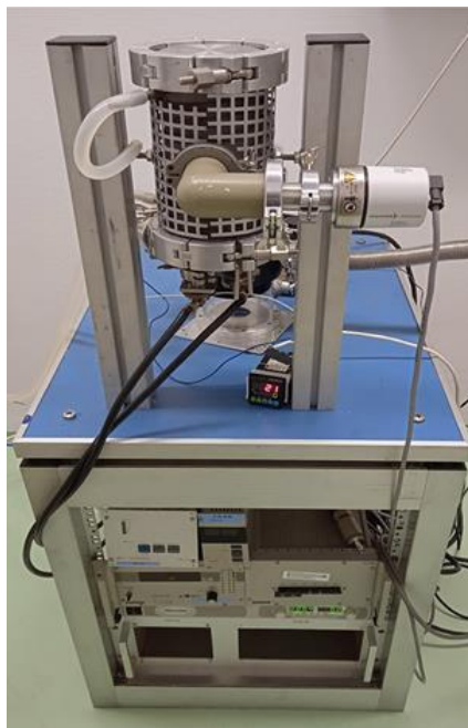
Figure 6. Photograph of the preliminary radionuclide separation equipment (RSE).
