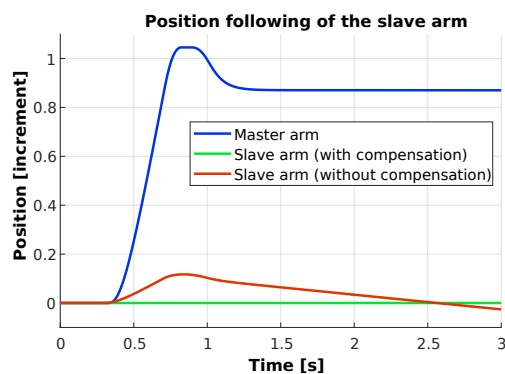
Figure 17: The same parameters applied to the slave arm failed to yield results.
