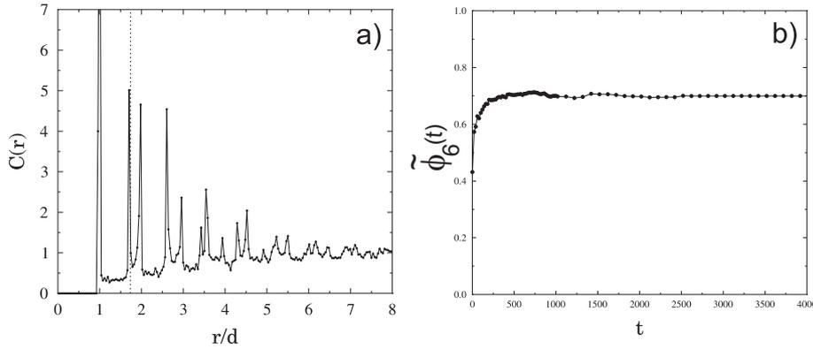
7.8. Figure: The density-density correlation function  $C(r)$  (a) and the bond orientation order parameter  $\tilde{\phi}_6(t)$  (b) were determined by computer simulations with  $N = 1000$  particles. Both quantities indicate a high degree of HCP order in the monolayer.
