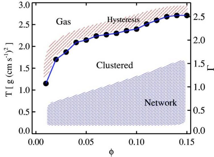
2.5. Figure: Phase diagram of a system of magnetized spheres which suffer dissipative collisions. The temperature of the system is controlled by externally imposed vibration. Typical structures of the “Clustered” phase are presented in Fig. 2.4.
