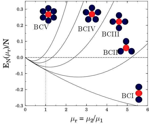
7.2. Figure: The energy Eq. (7.1) divided by the number of particles of basic configurations as a function of  $\mu_r$  for  $N = 3, 4, 5, 6, 7$ . For clarity, the corresponding particle configurations are also presented.
