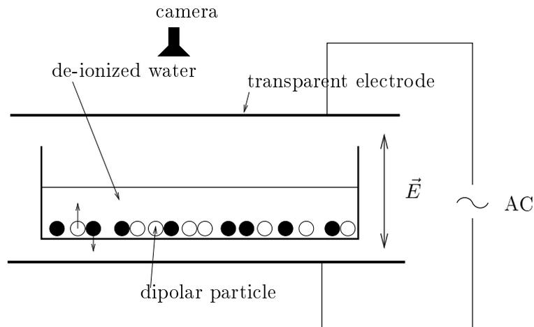
2.11. Figure: The experimental setup of Ref. [68] to study binary dipolar monolayers. The two sorts of particles sedimented to the bottom of the container. When a high frequency electric field was applied, the particles moved laterally and built up complex structures.
