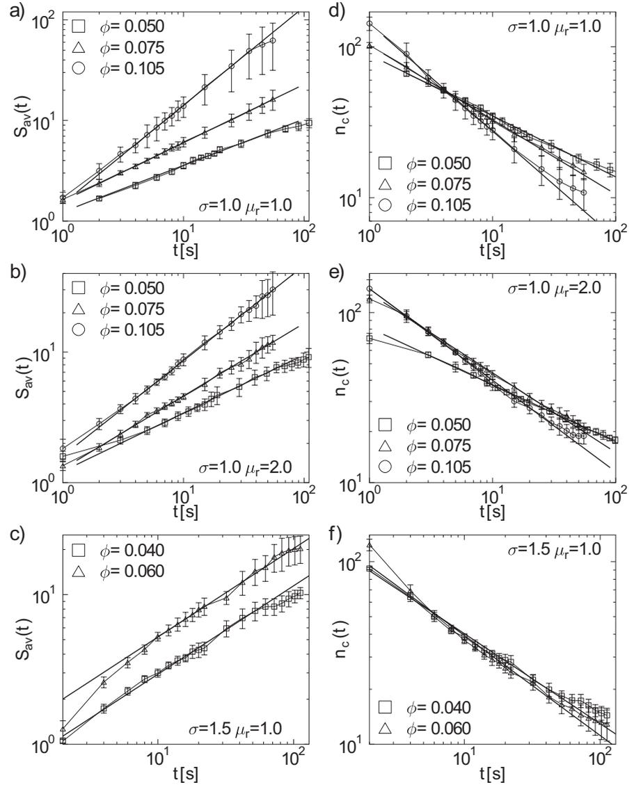
6.3. Figure: Average cluster size  $S_{av}$  (left column) and average number of clusters  $n_c$  (right column) as a function of time for the three experimental setups: (a), (d)  $\mu_r = 1$  and  $\sigma = 1$ , (b), (e)  $\mu_r = 2$  and  $\sigma = 1$  (c), (f)  $\mu_r = 1$  and  $\sigma = 1.5$ .
