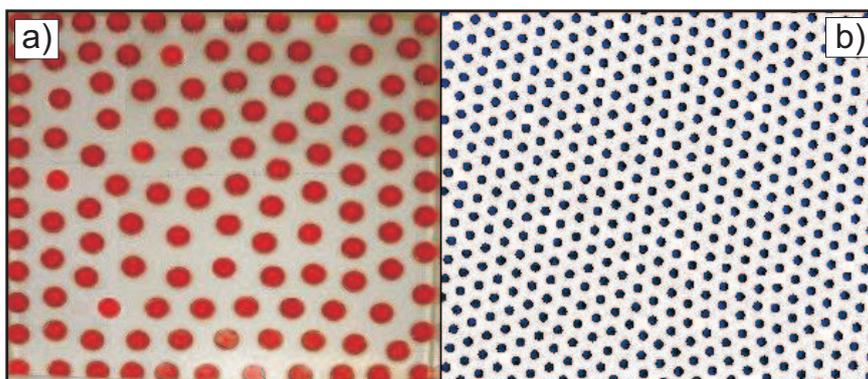
7.3. Figure: Triangular lattice of particles obtained for  $\phi_+ = 1$ ,  $\phi_- = 0$ . (a) In the experiments  $N = 100$  particles were used in a square-shaped container of side length  $L = 500$  mm. (b) Simulations were carried out with  $N = 500$  particles using periodic boundary conditions.
