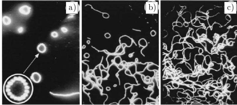
2.1. Figure: Clusters formed by dipolar particles in the absence of an external field varying the concentration. (a) At low concentrations the particles form chains and rings, (b, c) increasing the concentration more complex aggregates occur [100].
