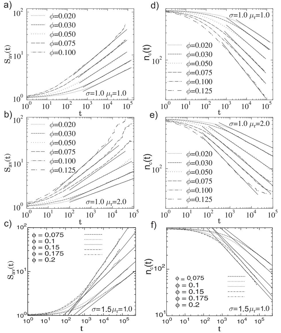
6.7. Figure: Average cluster size  $S_{av}$  (left column) and average number of clusters  $n_c$  (right column) as a function of time obtained by computer simulations of the three experimental setups.
