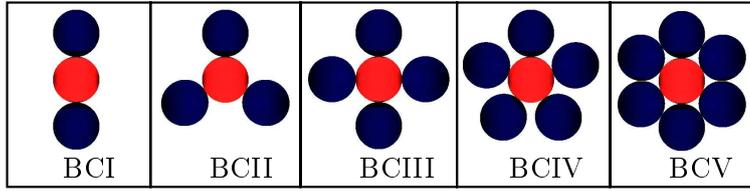
7.1. Figure: Basic configurations of BDMs. Particles are placed at the energetically most favorable location around an oppositely oriented dipole.
