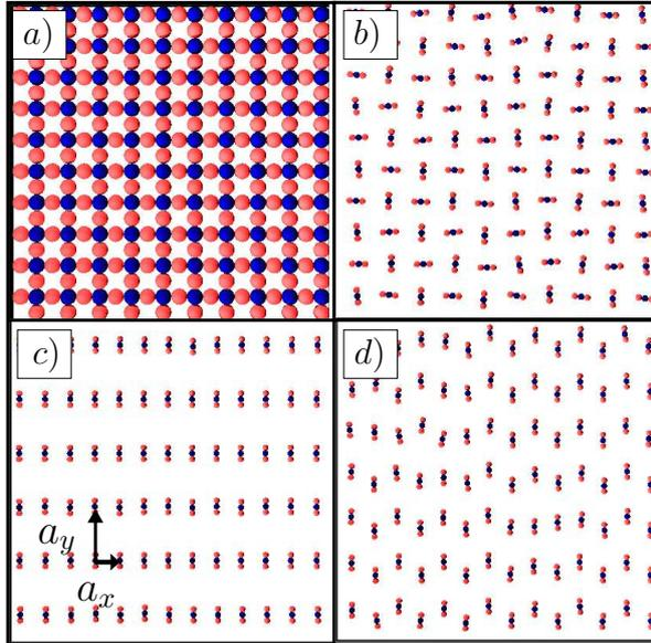
8.4. Figure: A bounded crystal of trimers with  $\mu_r = 1$ . (a) Molecular crystalline states of trimers obtained with  $\mu_r = 1$  at different values of the lattice spacings in the horizontal  $a_x$  and vertical direction  $a_y$ : (b)  $a_x = a_y = 5d$ , (c)  $a_x = 5d, a_y = 10d$ , and (d)  $a_x = 4d, a_y = 8d$ .
