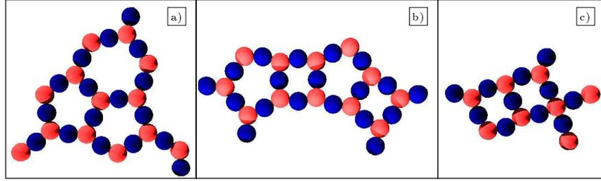
5.5. Figure: Net-like structures of polygons obtained by computer simulations with parameter values  $\mu_r = 2.0$ ,  $\phi_r = 1$ , and  $\phi = 0.125$ .
