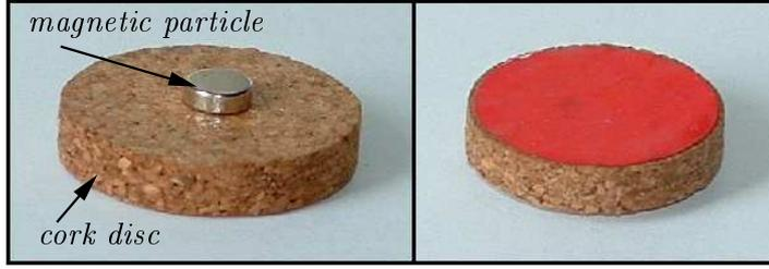
3.1. Figure: Magnetized particle attached to a cork disc of larger diameter (*left*). The composite particle can float upside down on the surface of water (*right*). The diameter  $d$  and height  $h$  values are  $d = 4$  mm and  $h = 1.5$  mm, and  $d = 26$  mm and  $h = 5$  mm, for the magnetic particle and cork disc, respectively.
