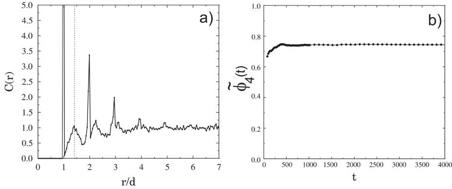
7.5. Figure: (a) The two-point correlation function presents well-defined peaks corresponding to the square lattice structure. (b) The bond orientational order parameter  $\tilde{\phi}_n$  calculated with  $n = 4$  takes a value close to 1, which indicates that a large fraction of the system has a square packed structure.
