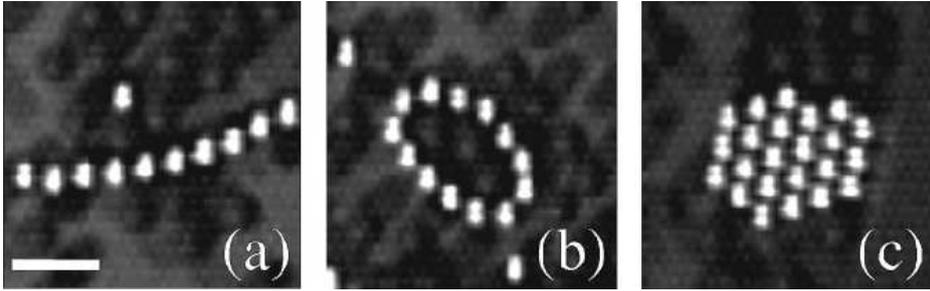
2.4. Figure: Examples of (a) chains, (b) rings, and (c) crystallites observed in an experiment where magnetized steel beads were vibrated in a container. The scale bar denotes 1 cm, the particle diameter was  $d = 3$  mm [7].
