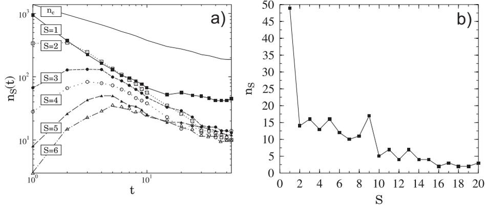
6.5. Figure: Cluster discrimination in BDMs obtained in setup (B). (a)  $n_S(t)$  for different cluster sizes  $S$  together with the total number of clusters  $n_c$ . (b) Number of clusters  $n_S$  of size  $S$  in the system at a given time  $t$ .
