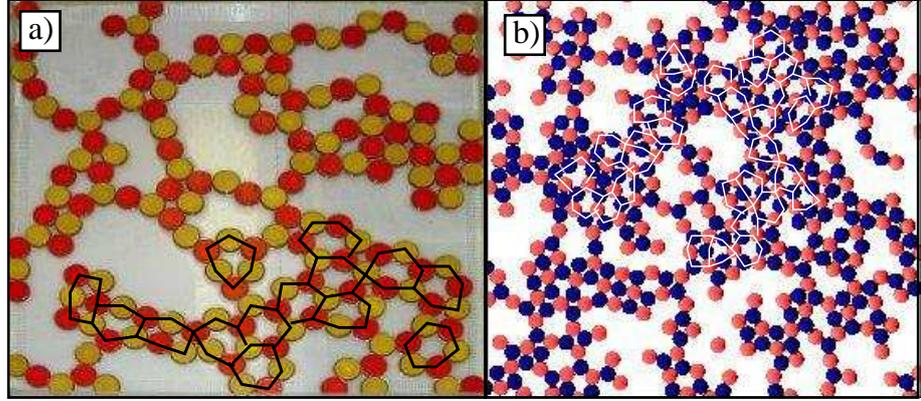
7.6. Figure: Honeycomb I lattice obtained by experiments (a) and computer simulations (b). For clarity, a few plaquettes of the crystalline structures are highlighted.
