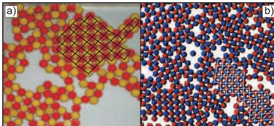
7.4. Figure: For the parameter values  $\mu_r = 1$ ,  $\phi_r = 1$  starting from a random initial configuration at high enough concentrations  $\phi$  the particles rapidly form an extended structure with square packed crystallites. For clarity, both in the experimental (a) and simulation results (b) we highlighted some plaquettes of the square lattice structure.
