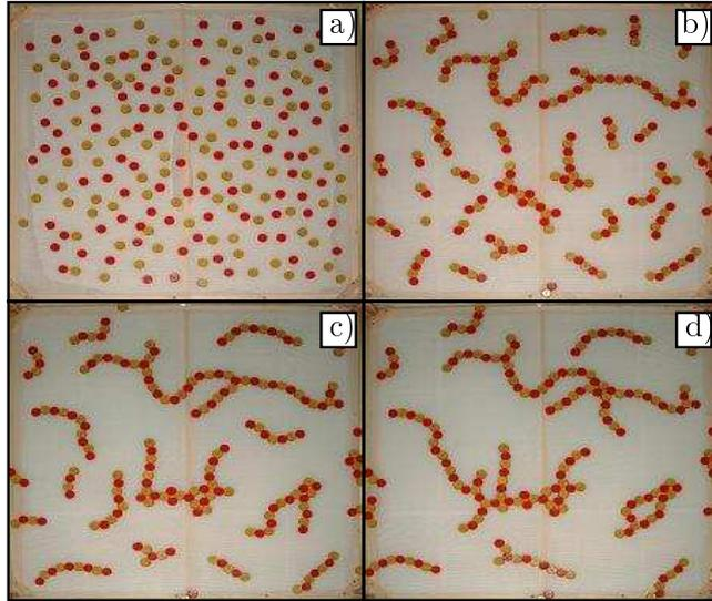
3.4. Figure: Representative example of the time evolution of the experimental system at a concentration  $\phi = 0.105$ . The relative dipole moment, polydispersity, and relative concentration of the components were set to  $\mu_r = 1$ ,  $\sigma = 1$ , and  $\phi_r = 1$ , respectively. The total duration of the experiment was 60 s, snapshots were taken at time values a)  $t = 0s$ , b)  $t = 10s$ , c)  $t = 30s$ , d)  $t = 60s$ .
