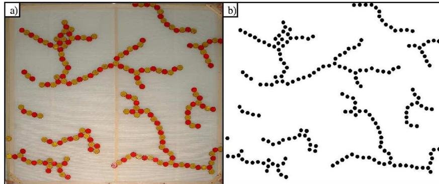
3.5. Figure: For the digital image processing GIMP was used throughout the experiments. In the original snapshot (*a*) black dots were placed on the particles from which a black-and-white image was generated (*b*). We worked out a cluster searching computer program which identifies connected sets of particles.
