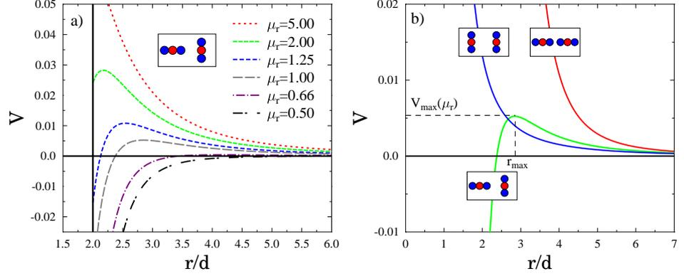
8.2. Figure: (a) Interaction of trimers with a fixed relative orientation  $\alpha_1 = 0$ ,  $\alpha_2 = \pi/2$  as a function of  $r$  for several values of  $\mu_r$ . (b)  $V(r)$  for different relative orientations at  $\mu_r = 1.0$ . For the case of perpendicular orientation a potential barrier exists with height  $V_{\max}$  and location  $r_{\max}$ .
