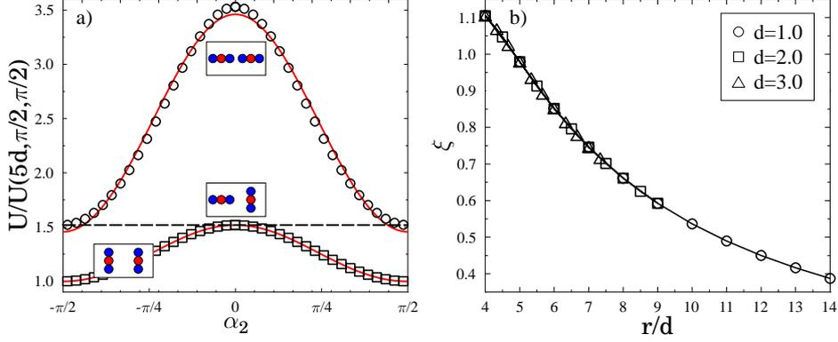
8.3. Figure: (a) Angular dependence of the interaction of trimers placed at a distance  $r = 5d$  with  $\mu_r = 1.0$ . The value of  $\alpha_1$  was fixed to 0 and  $\pi/2$  for the upper and lower curves, respectively, while  $\alpha_2$  was varied. The symbols show the numerical results, while the continuous lines were obtained by fitting with Eq. (8.1). (b) The parameter  $\xi$  of the angular component of the interaction potential as a function of  $r/d$ .
