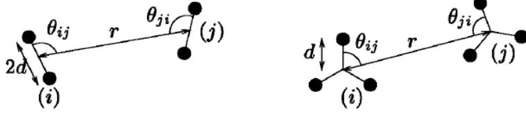
2.8. Figure: Definition of the notations adopted to compute dimer (*left*) and trimer (*right*) interaction. The black dots show the colloids and the line between them is a guide to the eye [1].
