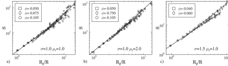
6.2. Figure:  $S(R_g)$  obtained in experiments for the three experimental setups. The slopes of the fitted straight lines  $D_1$  and  $D_2$  are summarized in Table 6.1.
