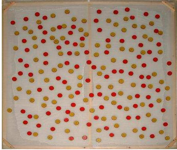
3.2. Figure: Initial configuration of 198 particles in a square box of side length  $L = 1000$  mm resulting in a concentration  $\phi \approx 0.1$ . The same amount of particles of opposite magnetic moment/different colors is used so that  $\phi_r = 1$ .
