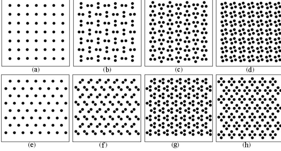
2.7. Figure: The colloid configurations (black dots) at  $T = 0.0$  for a square 2D periodic substrate (a)  $N_c = N_m$ , (b)  $N_c = 2N_m$ , (c)  $N_c = 3N_m$ , (d)  $N_c = 4N_m$  and for a triangle substrate (e)  $N_c = N_m$ , (f)  $N_c = 2N_m$ , (g)  $N_c = 3N_m$  (h)  $N_c = 4N_m$  [66].
