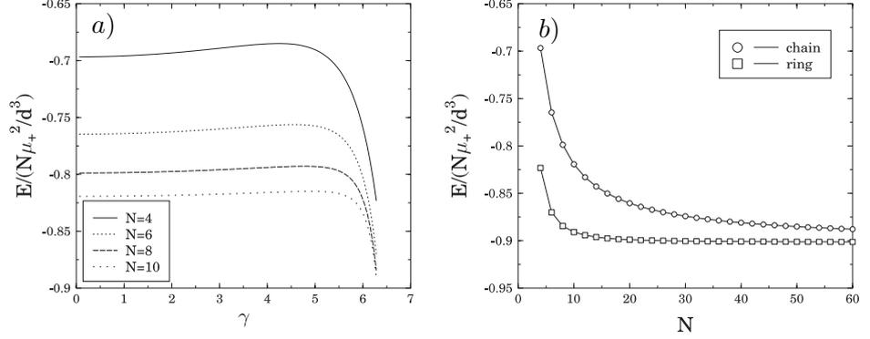
5.3. Figure: (a) Energy divided by the number of particles of a bent chain for  $N = 4, 6, 8, 10$ .  $E_{ch}(\gamma = 0)$  and  $E_{ch}(\gamma = 2\pi)$  provide the energy of a straight chain and a perfect ring, respectively. (b) Comparison of chain and ring energies as a function of the number of particles  $N$ . The energy difference of the two configurations disappears as  $N$  increases.
