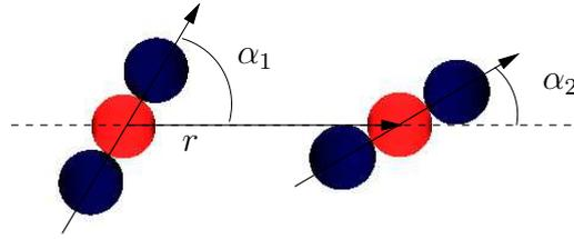
8.1. Figure: The relative position and orientation of trimers (BCI) characterized by the center-to-center distance  $r$  and the two angles  $\alpha_1$  and  $\alpha_2$ .
