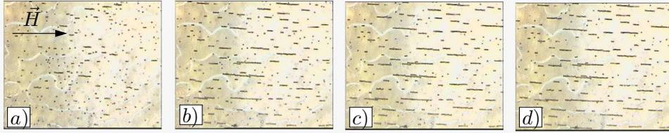
2.2. Figure: Experimental examples for the aggregation of permanent dipoles in a homogeneous external magnetic field. Initially the particles were randomly dispersed on the liquid surface. Then the particles aggregate (a) and form short chains which join into longer and longer chains (b, c, d) aligned with the field  $\vec{H}$ .
