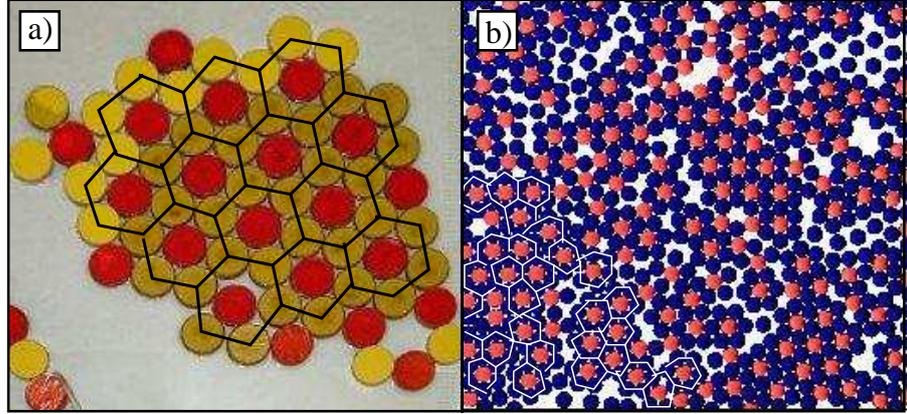
7.7. Figure: At large enough relative concentrations and relative dipole moments the system rapidly orders into the Honeycomb II lattice. Experiments (a) and computer simulations (b) are in a good agreement.
