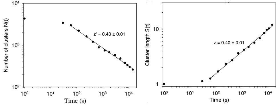
2.3. Figure: Example for the time evolution of the average number of clusters (a) and average cluster size (b) in an ensemble of particles with permanent dipole moment subject to a homogeneous external magnetic field [11]. The power law behavior can clearly be observed. The dynamic exponents  $Z$  and  $Z'$  are nearly equal.
