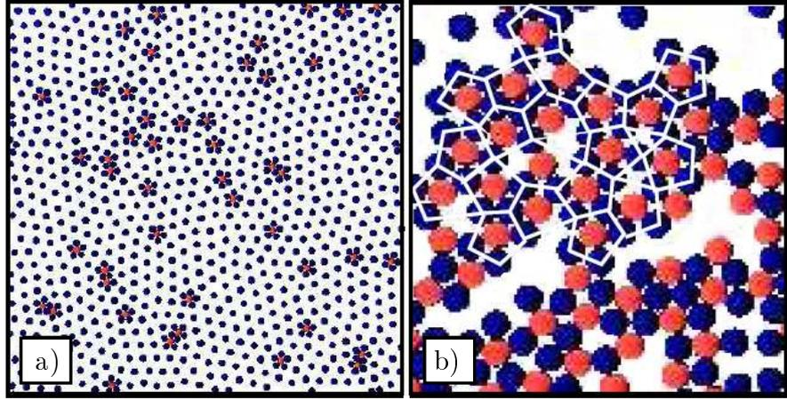
7.9. Figure: (a) Flower-like islands in a triangular lattice obtained by computer simulations at the parameter values  $\phi = 0.5$ ,  $\phi_r = 5$ ,  $\mu_r = 2.0$ . (b) Quasi crystalline structure with local five fold symmetry ( $\phi = 0.66$ ,  $\phi_r = 2$ ,  $\mu_r = 1.8$ ).
