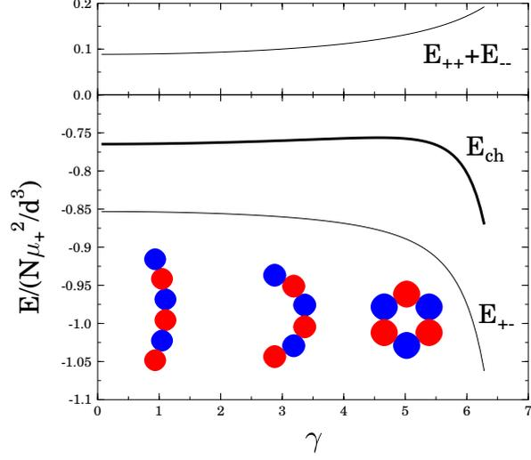
5.1. Figure: Energy of a bent chain divided by the number of particles as a function of the bending angle  $\gamma$  obtained from Eq. (5.5) for  $N = 6$ . For clarity, the particle configurations are also shown for  $\gamma = 1, \pi, 2\pi$ .
