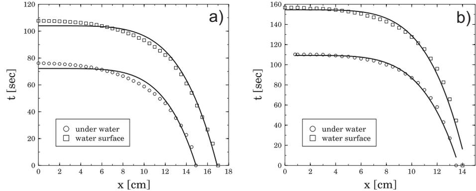
3.3. Figure: The time  $t$  as a function of distance  $x$  measured during the motion of a magnetic particle: (a) prolate particle with extensions  $d = 2$  mm and  $h = 6$  mm, and (b) oblate magnetic particle of diameter  $d = 4.0$  mm and height  $h = 1.5$  mm attached to a cork disc. The solid lines show the best fits obtained with Eq. (3.6) for both moving on and under the water surface.
