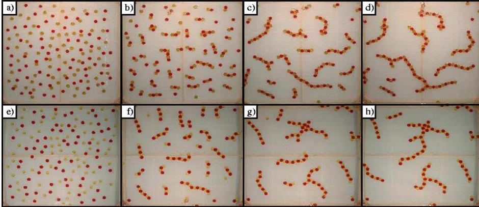
6.1. Figure: The time evolution of cluster-cluster aggregation for setup (A) ( $a, b, c, d$ ) at the concentration  $\phi = 7.5\%$  and for setup (C) ( $e, f, g, h$ ) at  $\phi = 6.0\%$ . Starting from the random initial configuration ( $a, e$ ) first single particles aggregate and form short chains ( $b, f$ ), which then merge resulting in large branching structures ( $c, d, g, h$ ).
