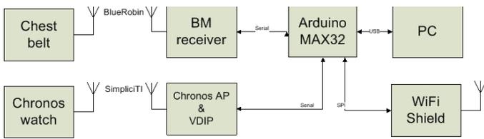
Fig. 1 Experimental platform schematics
