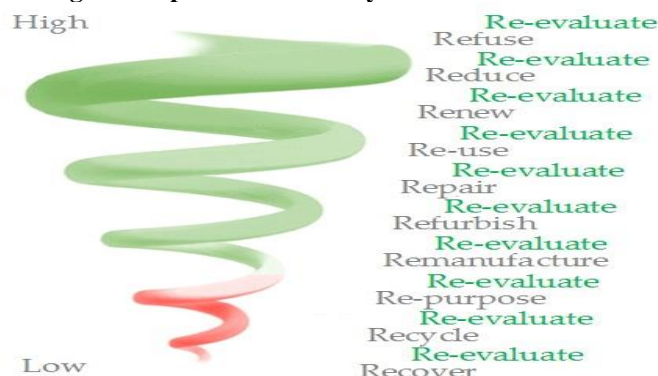
Figure 4. Spiral of circularity levels 10+1 r
