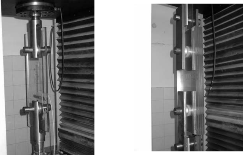
Figs. 9-10 Toughened glass specimens, 1 ply and 4 ply laminated glass
