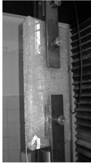
Figs. 11-12 Toughened glass specimens, 1 ply and 4 ply laminated glass pane after testing
