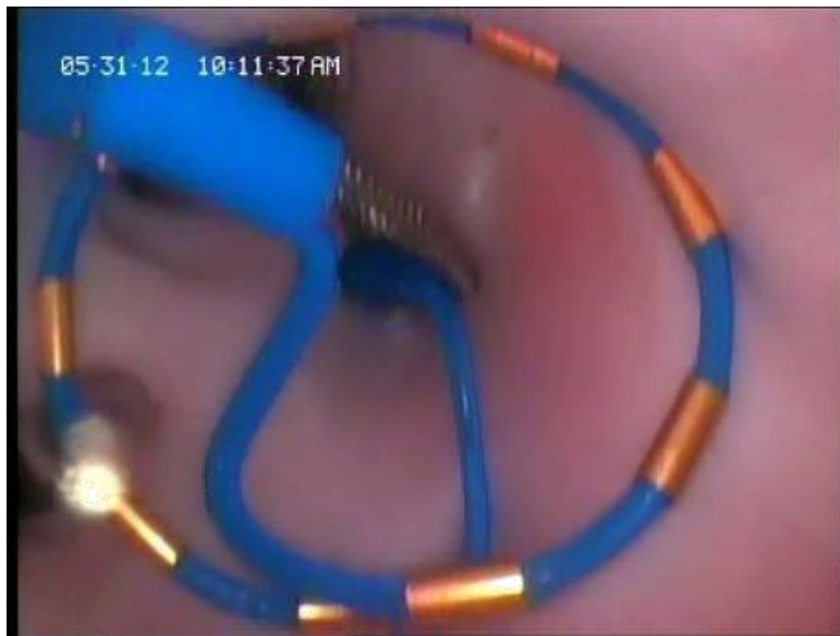
Figure 4. Electrodes 1 and 10 touching each other due to a squeezed circular segment of the catheter (intraatrial video frame from a cadaver heart, courtesy: Dr. Csanadi and Medtronic Inc).
