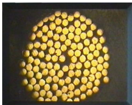
Fig. 6. 45° sharp-edged MEA consisting of 128, 100 \mu\text{m} diameter units (Own Photo)
