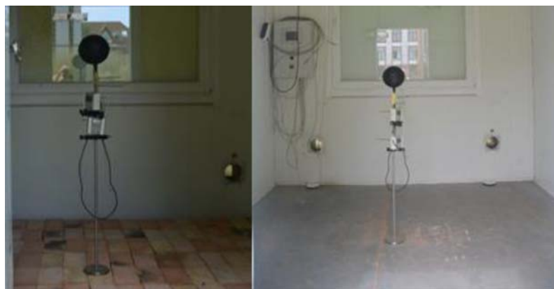
Fig. 2. PASSOL Laboratory with and without heat storage mass
