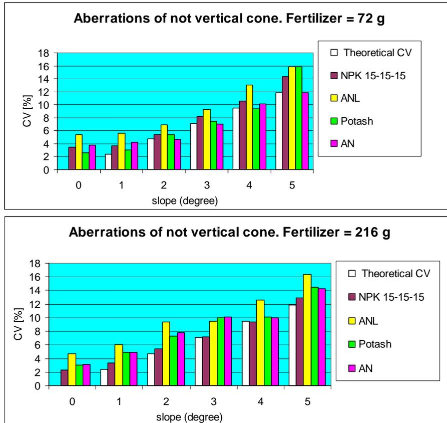
Figure 4: Result of examination the cone-belt dispenser
