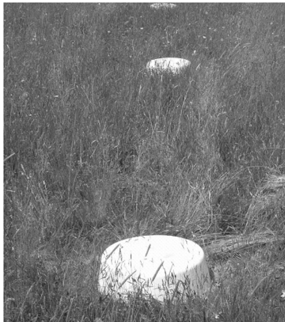
Figure 8: Application of the frame+bowl method in a grassland experiment
