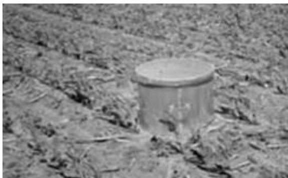
Figure 1: Simple plastic chamber for the delimitation of the measurement area
