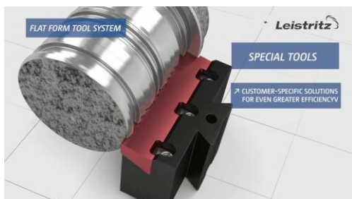
Fig. 1. The application of the flat form tool [4]
