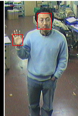
Figure 5: Localization of hand and face
