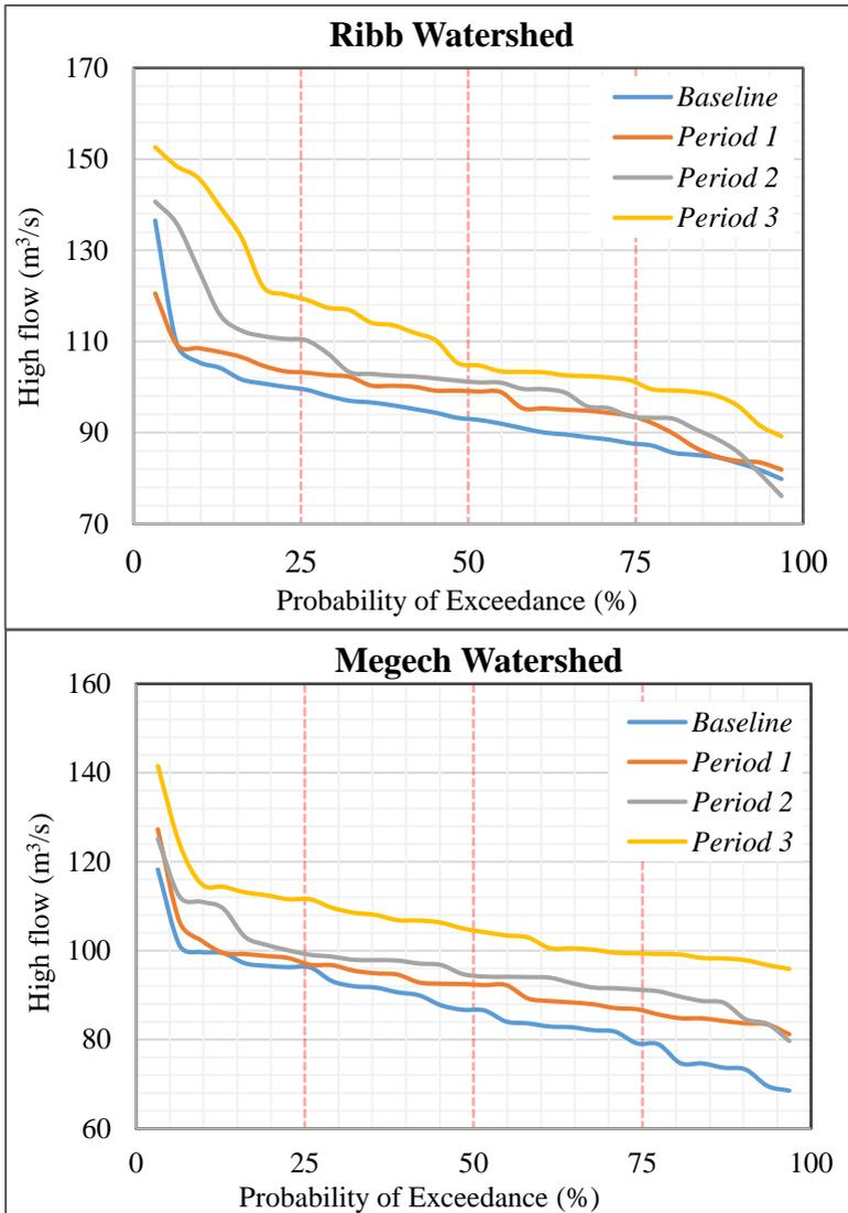
Figure. 8: Flow Duration Curve of High flows of Ribb and Megech watersheds
