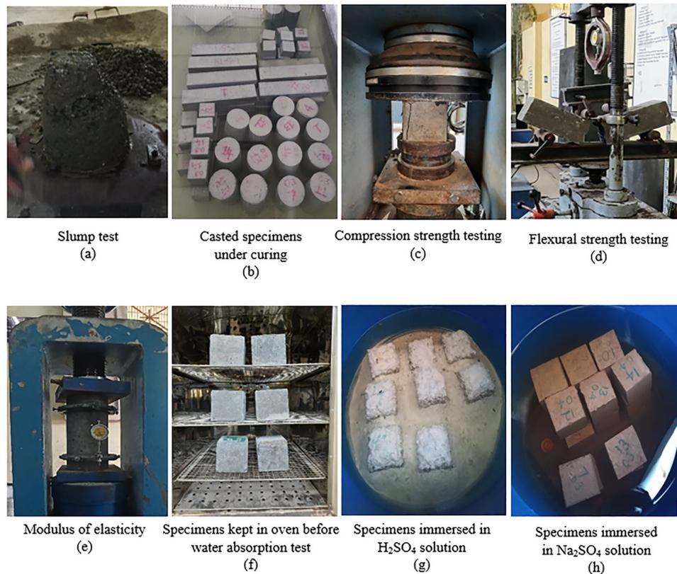
Fig. 2. Casting and testing of concrete specimens
